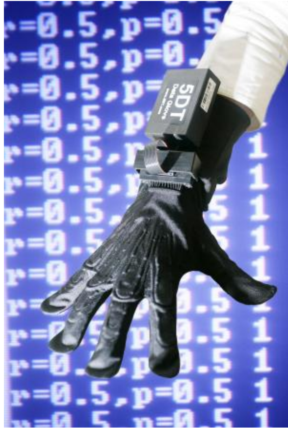
The 'cyberglove' used to capture data about how the human hand moves. (Credit: Image courtesy of University Of Portsmouth)
